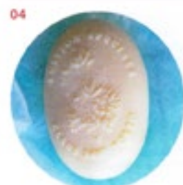
04 Stamp of approval Soap goes through a mould, is cut into bars and then impressed with a logo on a stamp at -15C.
