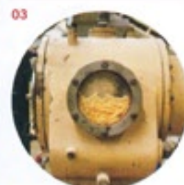
03 Refining Soap goes through another refiner, heated to 70C and then moves through a vacuum chamber to remove trapped air.
